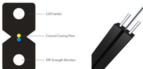
Indoor drop cable structure
